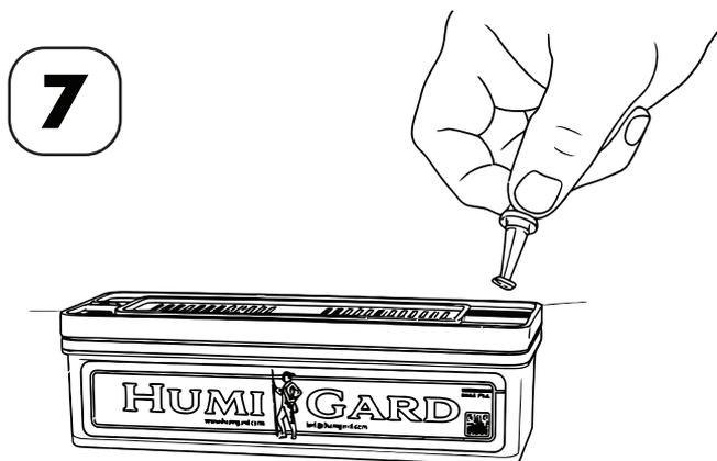
Replace the Fluid Filler Plug with a quarter turn (finger tighten only).
