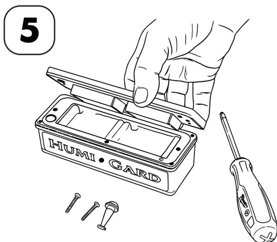
Replace the top vent and replace the screws (use a screw driver only, do not use a screw gun).
