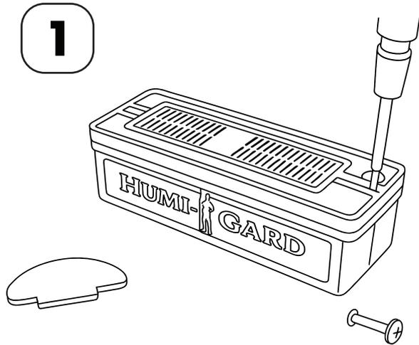
Remove the Filler Plug first (1/4 Turn by hand). Then remove the screws.
