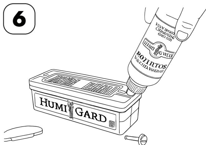
Fill the tank, no higher than the max fill line, **using only Cedar Cigar Fluid.**
