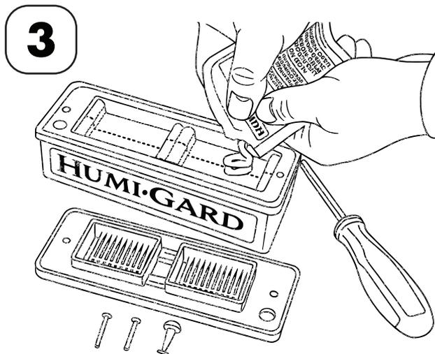
Select the evaporation paste you wish to use (Red 64-65%, Yellow 67-68%, Blue 70-71%). There are two packets for every color and you may need both. Cut off the corner with a pair of scissors, and fill both top trays of the Evaporation Chamber.
