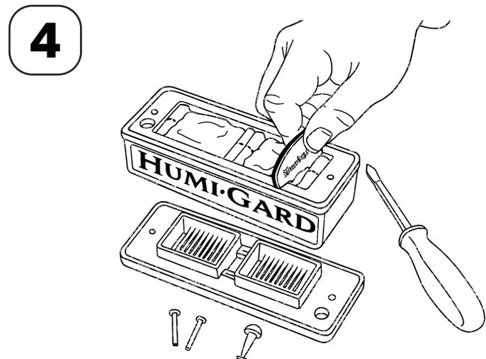
Use the Trowel provided to set the paste to the right depth. You can move paste from one side to the other, if necessary, to make sure both sides cover the wick evenly.
